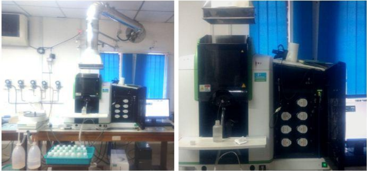
Figure 2.16: Atomic absorption spectrophotometer used in measuring heavy metals in ambient air sample.
