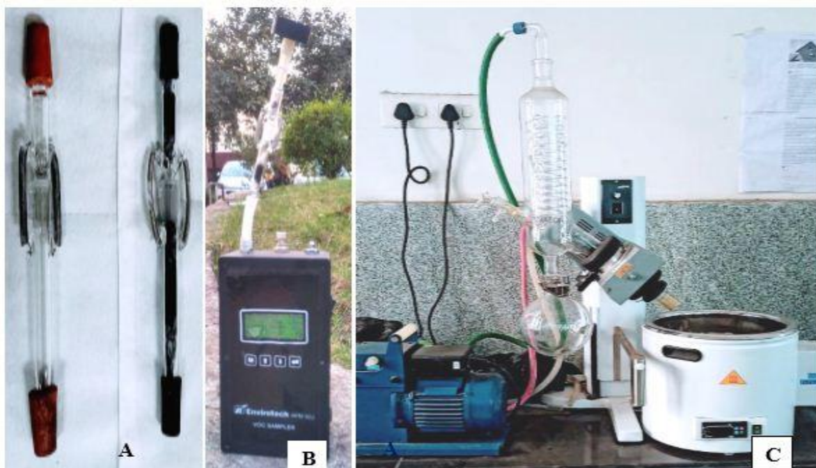
Figure 2.14: [A] Charcoal tube or VOCs sampling tube. Both empty [L.H.S.] and activated charcoal filled [R.H.S.] tubes are shown side by side; [B] VOC sampler and [C] Rotary vacuum evaporator to concentrate the VOC extract in CS 2 solution.
