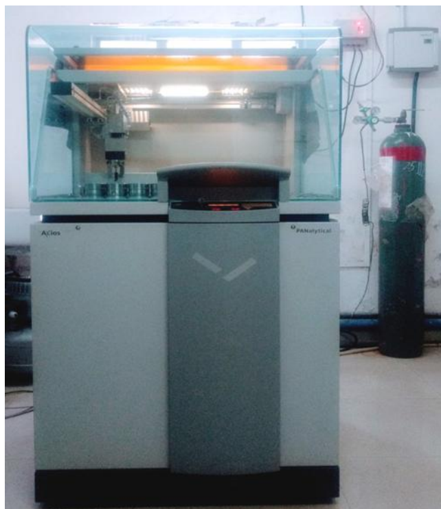
Figure 4.1: X-ray fluorescence spectrometer used for soil analysis.
