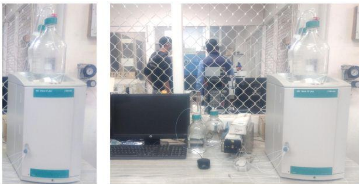
Figure 2.17: Ion–chromatography for poly-atomic ions measurement.
